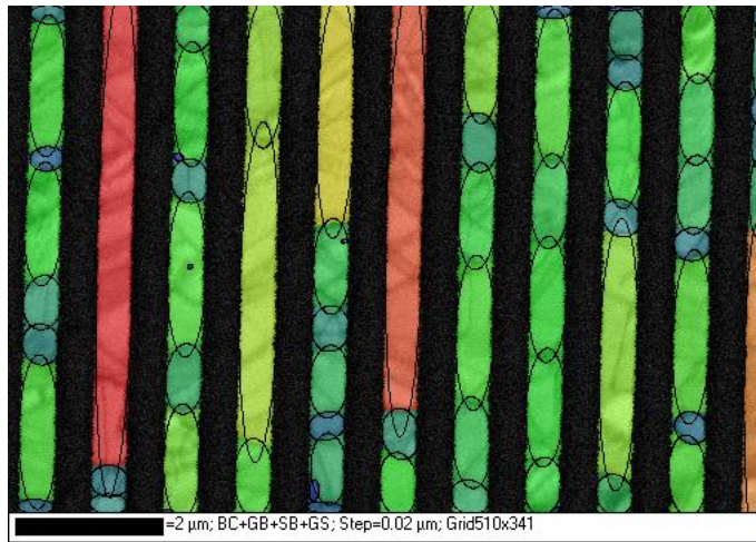
Grain map of 500nm Cu interconnects, showing best fit ellipses
